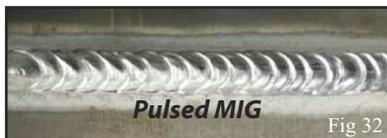
3. Welding with the use of the MIG/MAG method with double pulse causes smaller deformations than the traditional MIG welding
