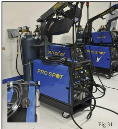
2. Welding with the use of the MIG/MAG method with double pulse achieves aesthetic standards as high as the TIG method (same look achieved with TIG welding)
