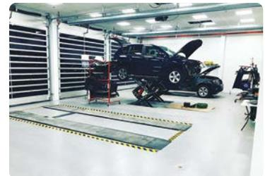
Pictured is the teardown section, where *Mountain View Auto* owner **Mike Daniels** said technicians disassemble 100% of the damaged area of the vehicle to create a repair plan.
