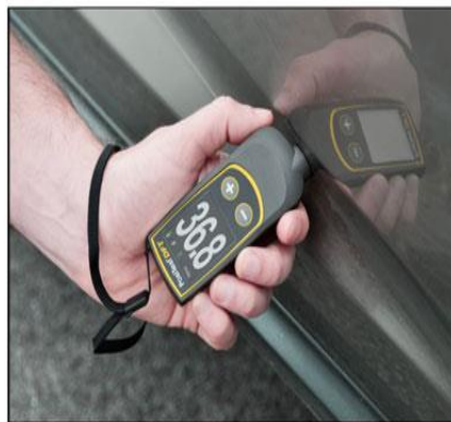
Figure D Significantly high readings indicate bodywork.
