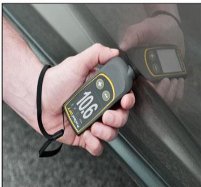
Figure C Higher readings indicate paintwork.
