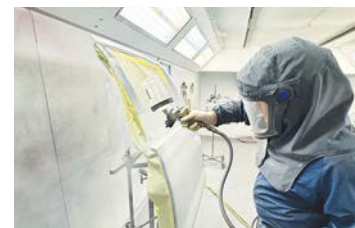
Spectrum Auto Body's painter, Walker, uses one of Spectrum Auto Body's SATA spray guns in the paint booth to achieve a clean, even finish. Shop owner Sam Brummund noted this isn't the new jet X, which only he uses.
