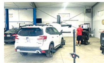
Technician Greg Doesher is shown performing a blind spot calibration on a Subaru Forester.
