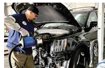
Daniel, sheet metal technician at JJH Auto Body & Paint, uses the Car-O-Liner® CTR9 Spot Welder during repairs.
