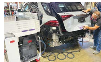
Mercedes-Benz Elite Certified Technician Gene Larson uses the 3M™ Clean Sanding System to prepare a liftgate repair.
