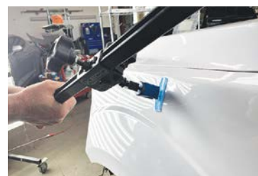
Shop owner Kenny Allen uses the KECO K-Bar tool to leverage out a dent.
