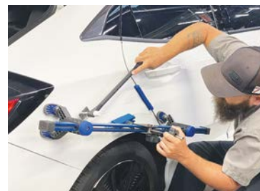
Repair technician Scott Burleson uses KECO's K-Beam to reshape the wheel opening body line. Prior to using the KECO GPR system, the technician would use stud welders to pull the dents, which could compromise the factory corrosion protection, or drill the panel, which could affect the vehicle's structural integrity.
