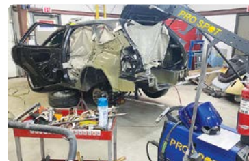
Having the latest equipment is essential to Dabler's success. Here, a damaged quarter panel is being replaced using a Pro Spot welder.
