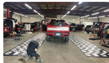
An investment in ADAS equipment, technician training and OE certifications enables Dabler Auto Body to exclusively service 2010 or newer vehicles equipped with ADAS. The 2020 Ford F-250 shown here is undergoing a post-repair calibration.
