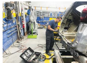
Annand Gaul uses Induction Innovations' Inductor Max. Noel said his once his shop's employees get the hang of induction heating tools, they prefer them to open-flame torches.
