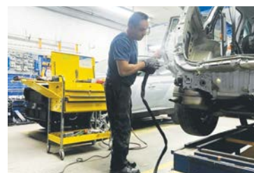
Noel said the induction heating tools from Induction Innovations are cleaner, safer and more versatile than traditional torches.
