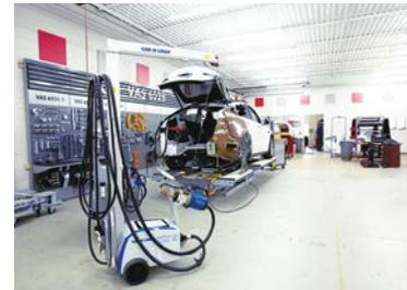
CARSTAR DANRICH uses several Car-O-Liner® OEM approved products, such as the Volkswagen 6528 Measuring and Alignment System, to repair damaged vehicles.
