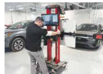
A technician positions the TruPoint system in line with the vehicle and confirms proper wheel alignment.
