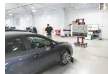
A technician performs a forward-facing camera calibration.
