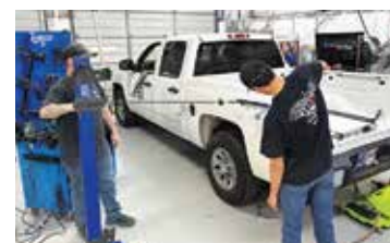
Techs Taylor and Ezequiel Chapina employ the KECO K-Tower, along with components and tools from the KECO L2E system, to repair a damaged bedside panel on a Chevrolet Silverado.
