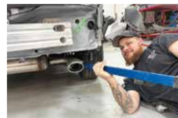
Master body technician Justin Taylor uses the KECO K-Power Lateral Tension Tool on the lower rear body section of a Toyota RAV4 to push the lower flange outward for a correction in panel alignment.
