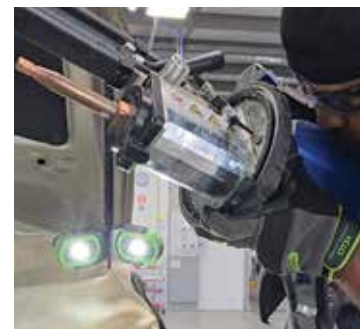
When it comes to following OEM specifications, Gasga Perez said the Car-O-Liner® CTR® 9 Spot Welder is an essential piece of equipment.
