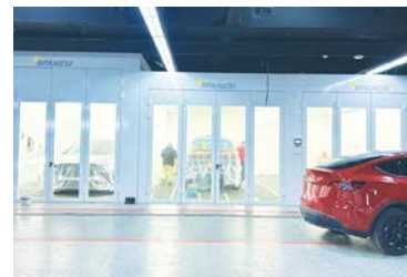
Among the Spanesi equipment at Richard's Body Shop are three custom designed spray booths, tailored for large vehicles like Rivian's Amazon electric delivery vans.
