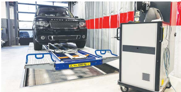
The Car-O-Tronic® Vision2 X3 and Car-O-Tronic® on the BenchRack™ help K & M Collision technicians return a Range Rover to pre-accident manufacturer regulations.
