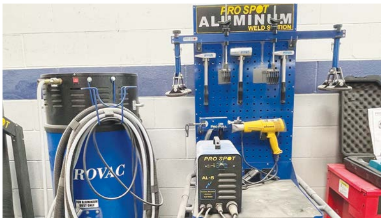
The Aluminum Weld Station includes a Pro Spot AL-5 Capacitor Discharge Stud Welder, designed for aluminum dent pulling to help repair a vehicle's panels. The equipment is especially helpful when working on trucks with an aluminum body, like the Ford F-Series.
