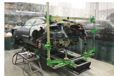
The damaged Aston Martin DB11 is mounted on a Globaljig frame machine, with additional fixtures attached for proper structural components replacement. The shop is Aston Martin-certified as a structural repair facility.
