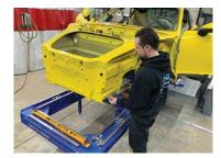
Technician Mike Krason is shown reassembling the front end of a 2020 Porsche 911 Carrera S. The severe structural damage required replacement of the entire front end. CCC® refers to the part as the front inner structure.
