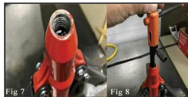
tightly, the threads are severely damaged and not repairable. In other words, a new rivet gun would have to be ordered. Kye used the internal thread restorer and was able to fix the gun. The kit was paid for with just one repair. See Figs 7-8
