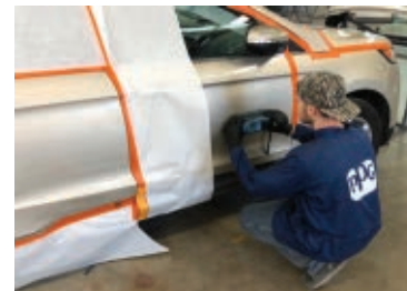
Painter Josh Van Wyngarden uses PPG's RAPIDMATCH® XI spectrophotometer to get dead-on matches at Pfeiffer Collision .
