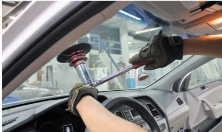
C&H Body Repair Inc. employee Jake Peters uses the Equalizer Viper, a device designed for small quarter glass removals, as well as windshields and back glasses.
