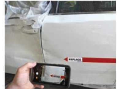
As a touch-less system, there's no need to write or attach anything to the vehicle's surface, thereby eliminating prep work.
