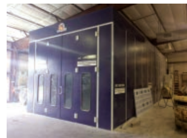
Foundation Ambulance invested in a 43'4" x 16'10" x 14'16" Accudraft booth that allows them to paint ambulances.
