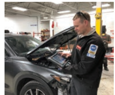
Master electronics and safety systems technician Paul Bostel uses the Autel scan tool to perform a pre-scan/blueprint scan on a vehicle at LaMettry's Collision .
