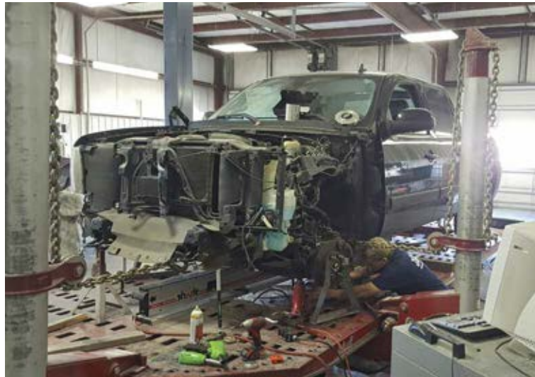
The technician finishes installing the Original One Part lower control arm and pulling the frame back to specifications, using an electronic measuring system.
