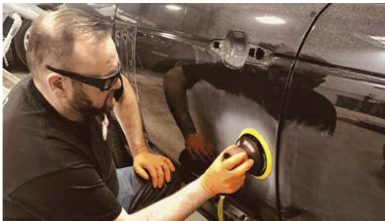
Florida Pneumatic's AIRCAT 6700-6-336 6-inch Orbital Palm Sander has a lubrication-free air motor.
