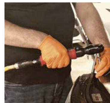
The AIRCAT 802 3/8 inch Composite Twin Pawl Ratchet has 90 ft-lb loosening torque and 280 RPM.
