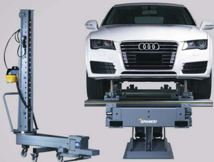
Spanesi's 106 Bench includes 10 ton pulling tower and our Universal Jig system (not shown)
